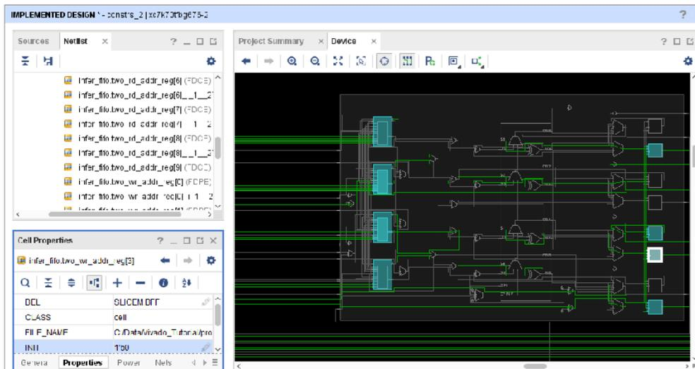
These properties can include everything from block RAM INITs to the clock modifying properties on MMCMs. There is also a special dialog box to set or modify INIT on LUT objects. This dialog box allows you to specify the LUT equation and have the tools determine the appropriate INIT.
