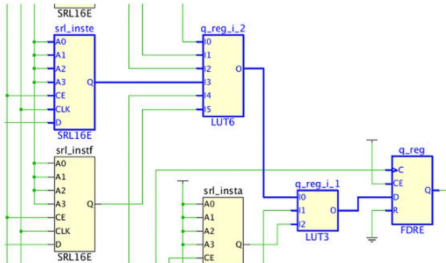
After shift register optimization, the final stage of the shift register is pulled from the SRL16E and placed in the logic fabric to improve timing, as shown in the following figure.
