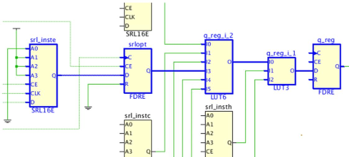
The `srl_inste` SRL16E address is decremented to reflect one fewer internal register stage. The original critical path is now shorter as the `srlopt` register is placed closer to the downstream cells and the FDRE cell has a relatively faster clock-to-output delay.
