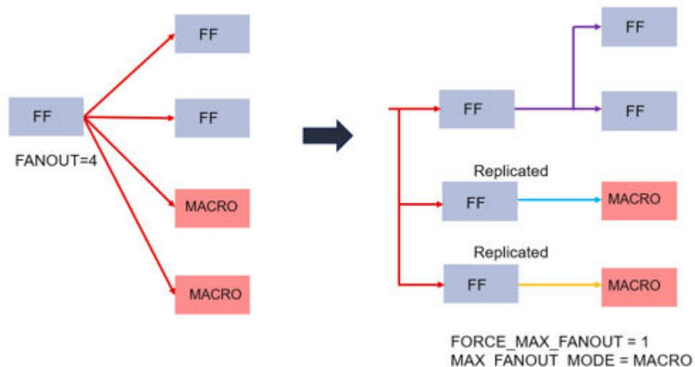
**Note:** This optimization happens early in the placer. In the later stages of the placer as the timing accuracy improves, both the replicated source and/or load registers may be moved to different clock regions or SLRs if the timing estimate improves.
