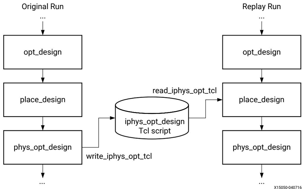
Two runs are involved, which are the “original run,” where `phys_opt_design` is run after `place_design` and the “replay run,” where `phys_opt_design` netlist changes are performed before placement.
