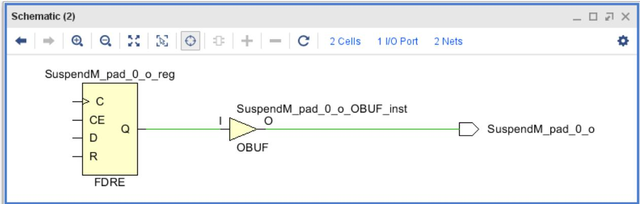
The following Tcl commands show how to add an inverter between the output of the FDRE and the OBUF:
