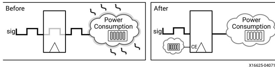
Intelligent clock gating also reduces power for dedicated block RAMs in either simple dual-port or true dual-port mode, as shown in the following figure.
