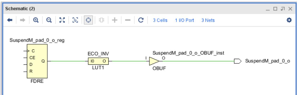
After the netlist has been successfully modified, the logical changes must be implemented. The LUT1 cell must be placed, and the nets to and from the cell routed. This must occur without modifying placement or routing of parts of the design that have not been modified. The Vivado implementation commands automatically use incremental mode when `place_design` is run on the modified netlist, and the log file reflects that by showing the Incremental Placement Summary:
